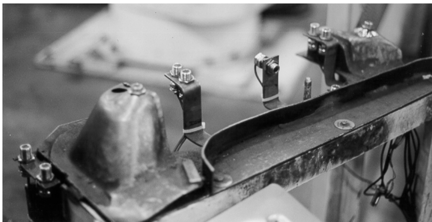
Figure 1. A welding fixture is modified by placing each sensors into a Quicktube™ mount. Use of Quicktubes prevent sensors from being damaged or destroyed due to impacts from parts.
